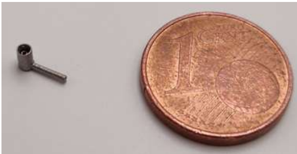
Figure 5 Micro kiel probe (D=1.6mm) - not extended
