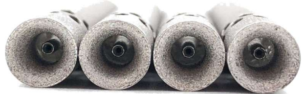
Figure 2 Kiel probes (front view)
